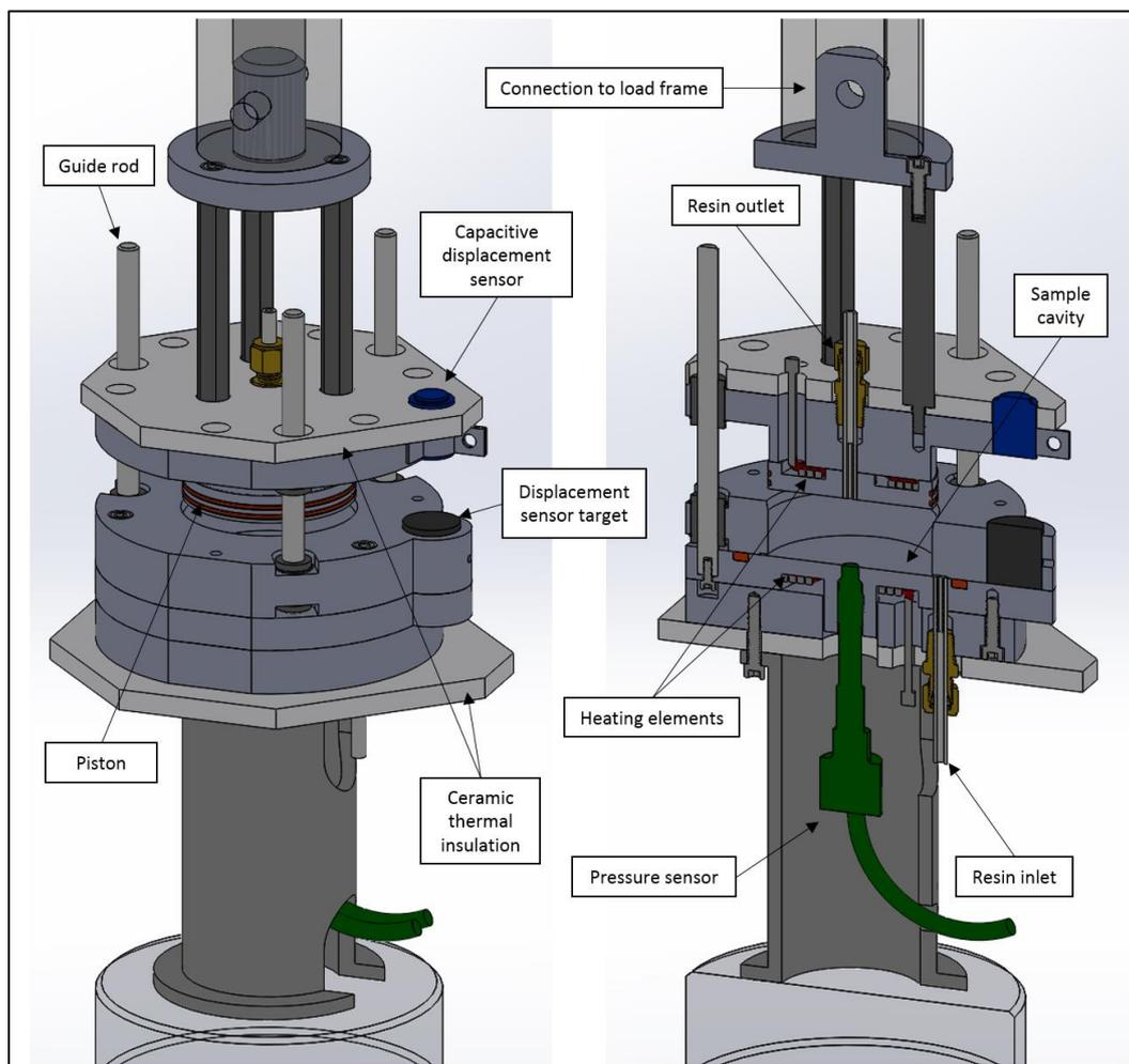
Figure 1: CAD model of the hybrid RTM/dilatometer tool.
